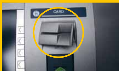
Device placed over card slot (example) Copies data from the magnetic strip
