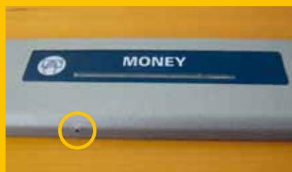
Mini camera (example) Films unprotected input of the PIN.
